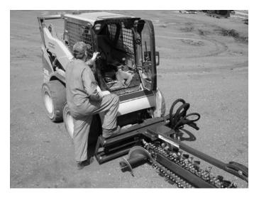
1. Use the step, safety treads, and grab handles to get on and off the loader and attachment.
