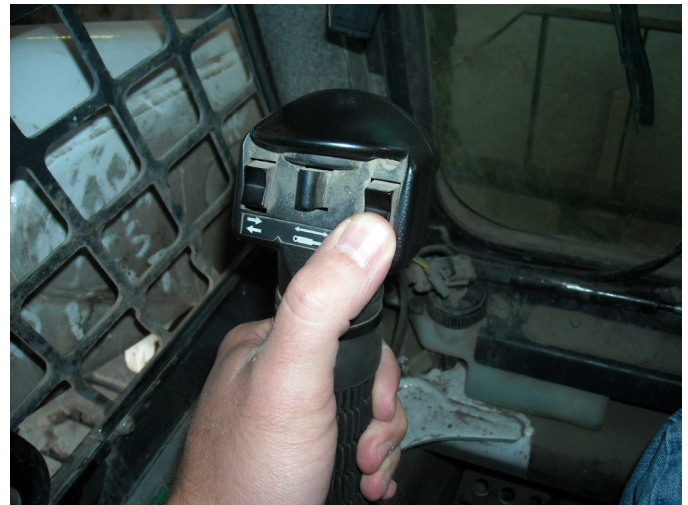
PUSH AND HOLD TO ENERGIZE DIVERTER
