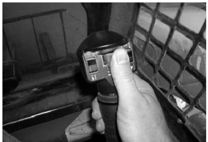
OPERATE AUX HYDRAULICS TO TILT
