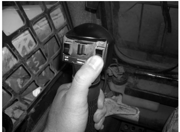
PUSH AND HOLD TO ENERGIZE DIVERTER
