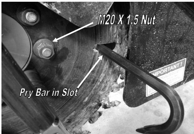
Cutter Head Lug Nut Removal
