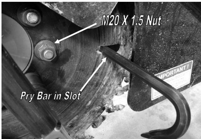
Cutter Head Lug Nut Removal
