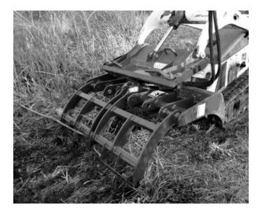
**A CAUTION** Always close the grapple securely before setting the attachment down on the ground. To avoid serious injury or death from crushing, NEVER put any body part near the grapple while open.
