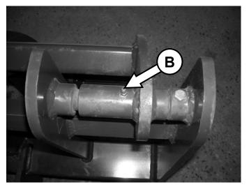
Grease the left, center, and right pivot pins **[B]** every **8 hours** of operation.
