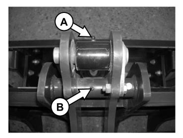
Use No. 2 lithium base grease gun when lubricating all attachment grease fittings.
