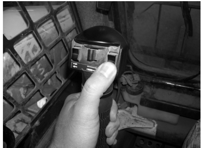
PUSH AND HOLD TO ENERGIZE DIVERTER
